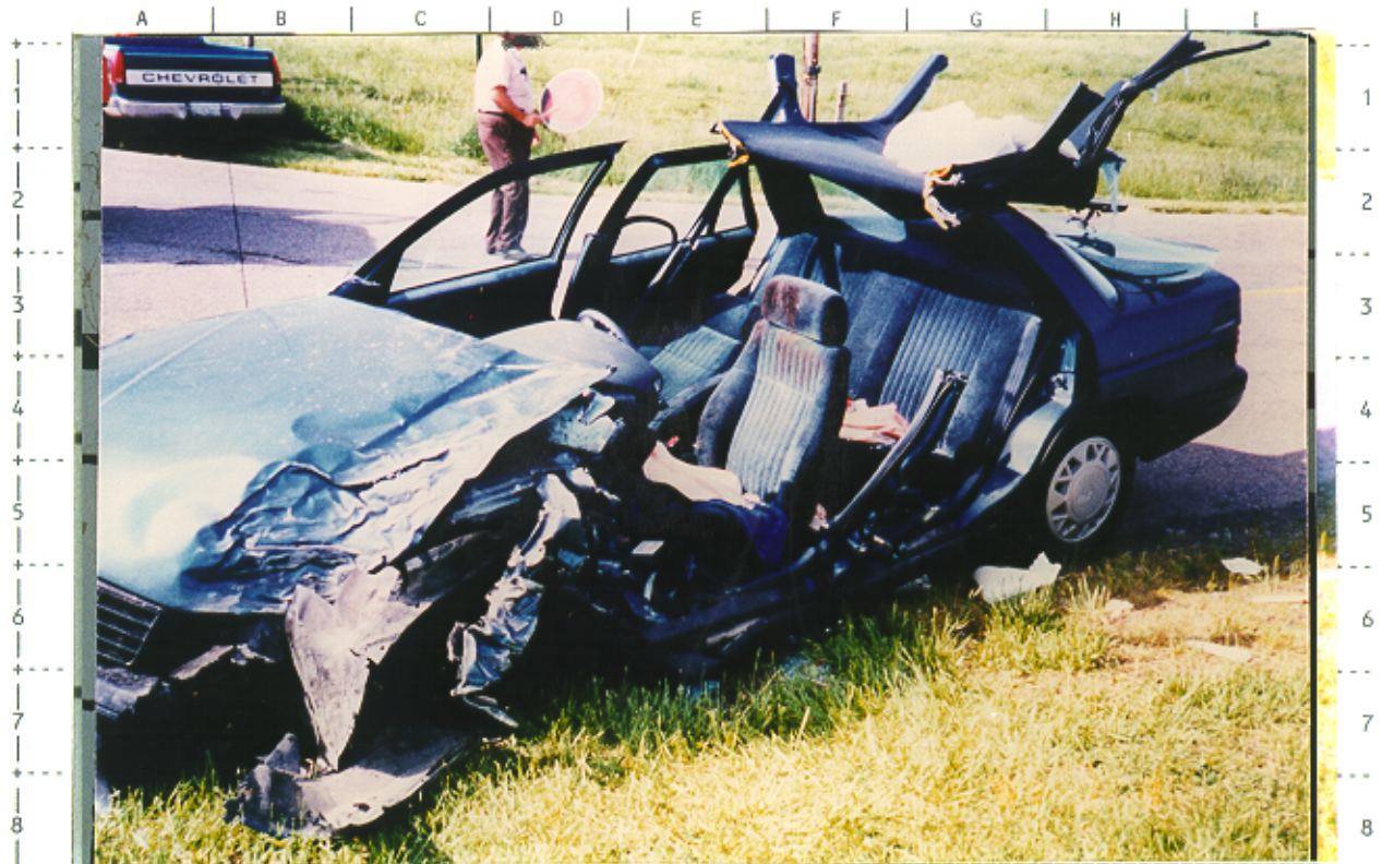
# 11 -- On-scene southwest view of 1991 Chevrolet Corsica at final rest after driver's extraction; NOTE: cut left B-pillar & blood
